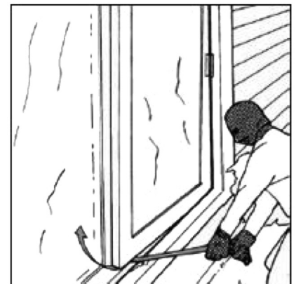
Figure 2 Rotating motion of the panel caused by prying action, can break the lock.
