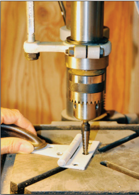
Enlarge two or more hinge holes using a stepped metal cutting drill bit.
