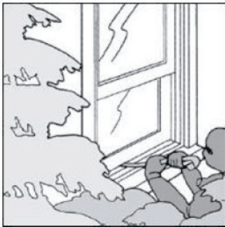
All windows within 6 1/2 feet of ground level should be burglar resistant. Also secure windows easily accessed from balconies, shade structures or low roofs.
